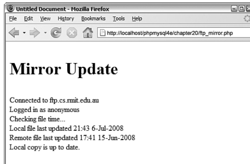
Figure 20.4 The FTP mirroring script checks whether the local version of a file is up to date and downloads a new version if not.
